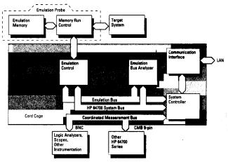
HP 64700 series emulators/analyzers have a dual-bus architecture. This dual-bus architecture gives you maximum transparency by allowing traces to be executed and displayed without halting processor execution.
