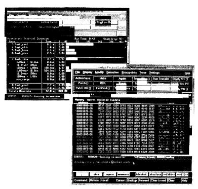
The graphical user interface combined with the HP Software Performance Analyzer provides a complete, real-time view of program execution.
