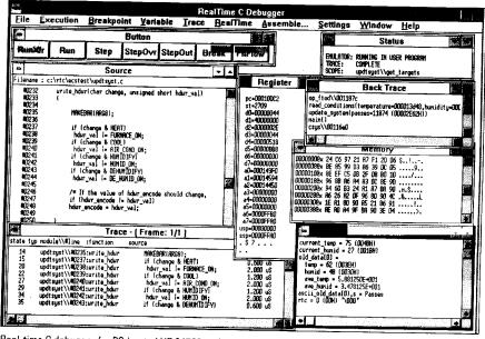
Real-time C debugger for PC-hosted HP 64700 series emulators offers powerful, nonintrusive debugging of embedded C and assembly code. Real-time concurrency allows several views to be active while a target system runs.
